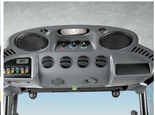
The heater and A/C controls are conveniently installed in the cabin roof.
