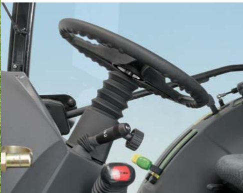
The steering wheel is adjustable in height, allowing every driver to find the ideal seat position.
